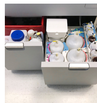
The continuous fluids/waste module is an in-lab upgrade to the Panther system.
